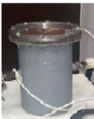
Fig. 2. Experimental model of pressure vessel with stratified cover [2]
